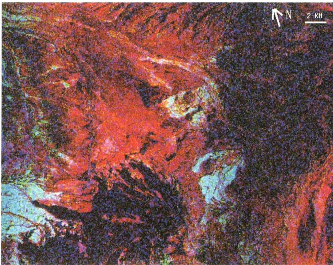
Plate 1. Composite red-green-blue interferometric coherence map constructed using three representative coherence maps as colors: 35-day coherence as the red channel, 1-year coherence data as the green channel, and 2-year coherence data as the blue channel. The image has the same dimensions as Figure 1. Green and blue colors represent regions that maintain good coherence over more than 1 year, which probably represent areas covered by lavas.
