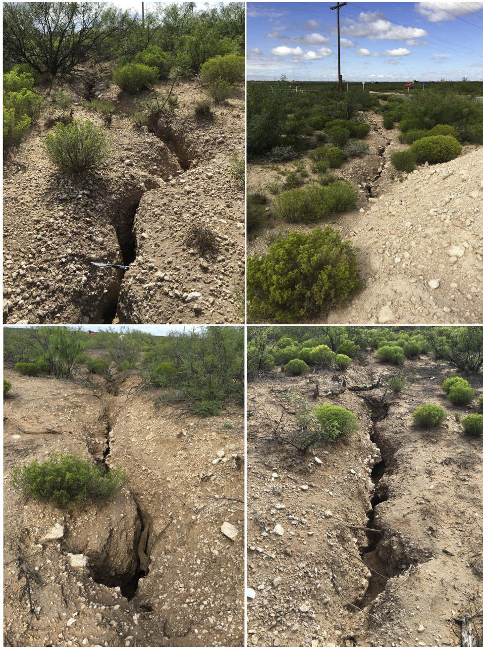
Fig. 11. Photos taken in September 2016 of ground fissures (light blue lines in Fig. 8(a)) found around the intersection of County Road 201 and 204 (region 'f' along profile \overline{AB} in Fig. 6(a)). The width of the fissures is \sim 10 cm. (For interpretation of the references to colour in this figure legend, the reader is referred to the web version of this article.)
