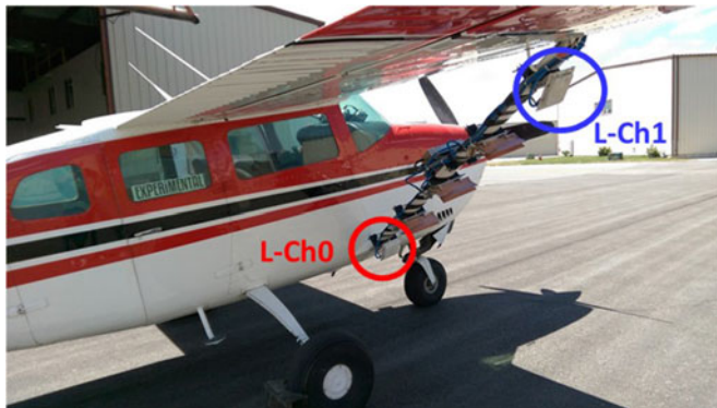
Fig. 2. Installation of the L -band antennas (at the very top and bottom) on the wing strut.
