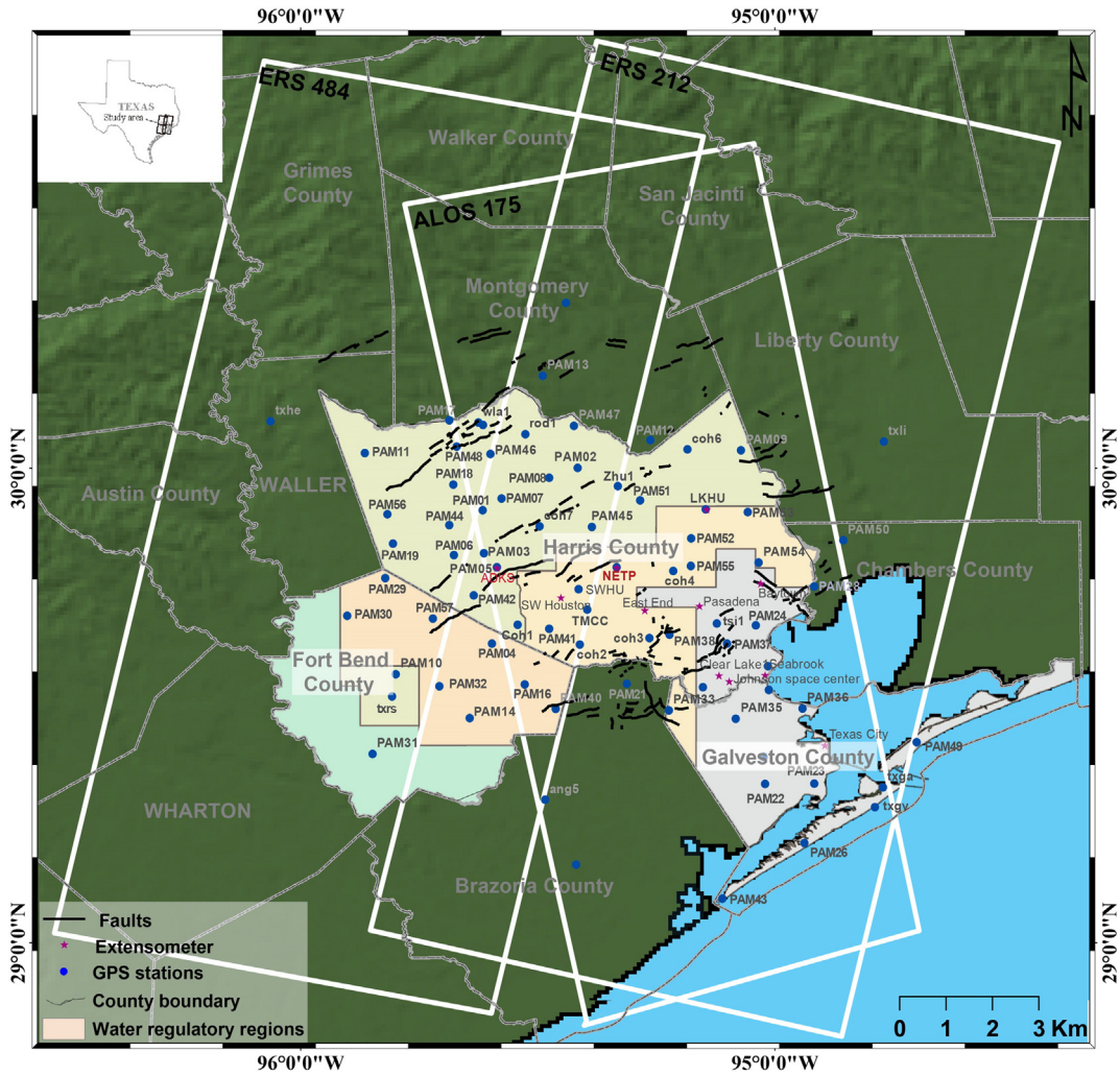
Fig. 1. Shaded relief map of Houston–Galveston, where faults (black lines) (Khan et al., 2014; Khan, 2014), GPS benchmarks (with prefix PAM and marked by blue dots), Extensometers (marked by pink stars), County boundaries and six ground water regulatory areas (by HGSD and FBSD) are superimposed. The ADKS and NETP are co-located extensometer/GPS stations, which are annotated in red. The GPS CORS station NETP is also used as the reference point in this study. The white rectangles represent the coverage of four SAR datasets used in this study. The map of Texas State is an inset on the upper-left corner.
