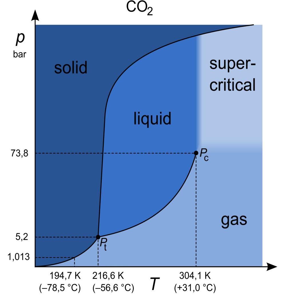
Carbon dioxide is the most commonly used supercritical solvent and the solvent of choice for the supercritical fluid extraction of lithium. Above is a phase diagram for carbon dioxide, showing the pressures and temperatures needed to reach a supercritical state. Below are pictures of the lab set up.
