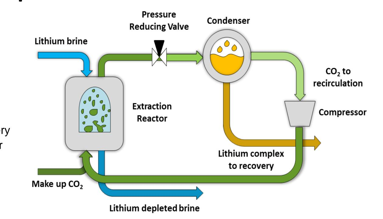
A fast and effective extraction process where the chemistry of the extractants and the pressure in the system are used for process control.
