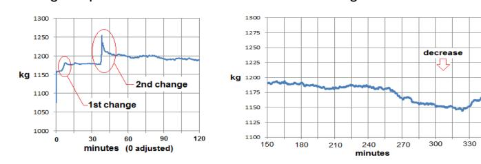
The '1st change' and '2nd change' area mark times when the well valve was closed slightly, choking the well and increasing the overall measured weight. This directly relates to a change in dryness fraction (x). The sensor can track changes in x of less than 1%. Note the 'decrease' seen late in the test. This is an effect that occurred from the well itself, and shows that the sensor can notify us immediately about changes occurring naturally in the well.
