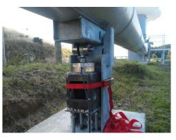
Load cells installed on two in-line supports allow the ability to measure the velocity of the water flow, which can be used to calculate the overall Mass flow Rate. A single load cell is sufficient to determine changes to dryness fraction (x), and changes to flow regime or detection of dangerous flows such as slug flow.
