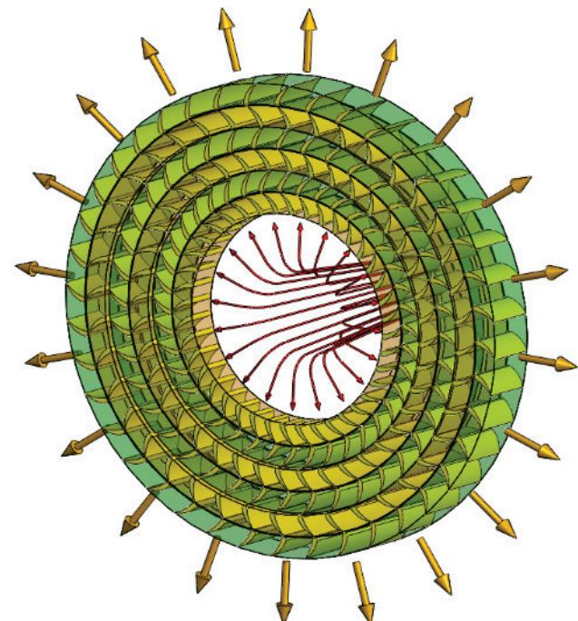
Only the Radial Outflow Turbine allows multiple pressure admissions on a single disk.
