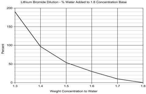
movement from the 1.8 concentration (utilized as the measurement base) to a concentration of 1.7 causes the addition of only 11% more water whereas the dilution from 1.4 to 1.3 requires a dilution of 90%. Overall there is absorption of 190% when
