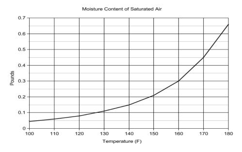
of elevated saturated air temperature range from 100°F to 180°F. At 100°F, for example, air has a saturated moisture content of approximately 0.04 pounds water per pound of air, while at 180°F, moisture content is 0.66 pounds.
