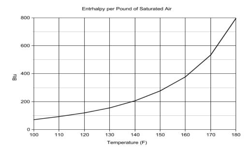
Upon reaching the desired temperature and enthalpy level as found in the upper ranges of the above charts, the saturated gas exits the heater / saturator and contacts a liquid desiccant which is a hydroscopic substance capable of removing moisture from the air stream in a dehumidification module. Removal of water from air in this context is an adiabatic process and in thermodynamics, an adiabatic process is one in which the specific enthalpy (energy) of the air remains constant.
