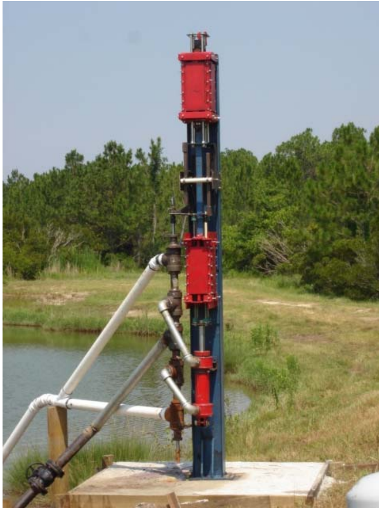
Linear Power, Ltd.'s Kinetic Energy Linear Alternator
