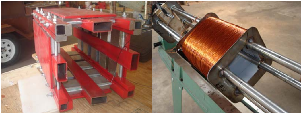
Shown above on the left are permanent magnets in a Housing and to the right a copper wire coil attached to non-magnetic stainless steel bars that drive the coil back-and-forth
