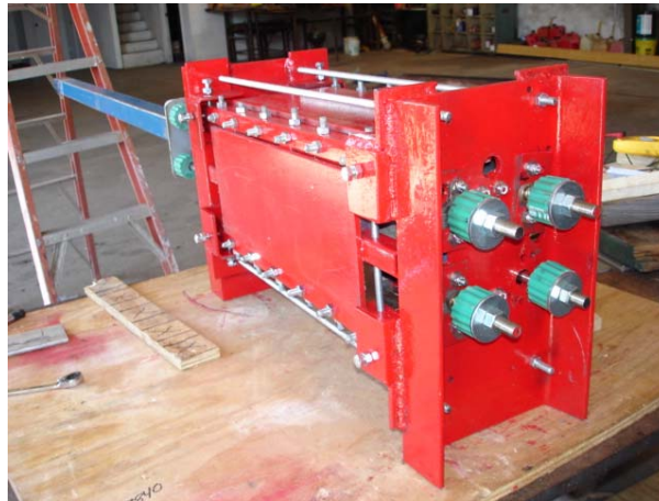
Linear Alternator developed by Linear Power, Ltd.
