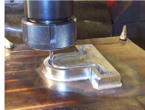
Making cooling channel
