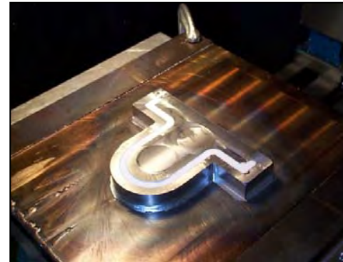
Support Structure for cooling channel
