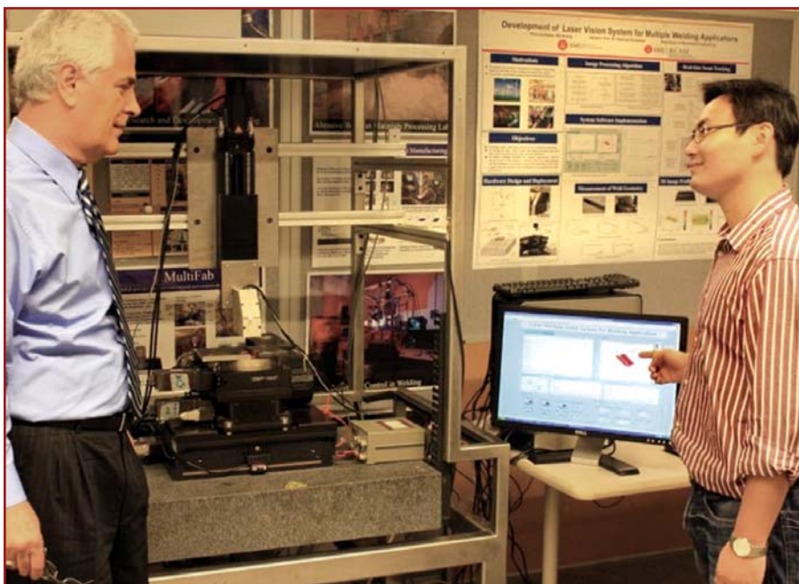
Fig. 4 — PhD candidate Wei Huang (right) explains to Dr. Kovacevic a newly developed laser-based machine vision system for joint tracking, adaptive fill control, and postweld inspection.
